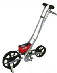
Earthway Seeders are a great first step to small scale mechanization. The light aluminum frame and plastic seed hopper makes it light, yet sturdy enough to withstand seasons of planting with proper care. The seeder comes with a variety of interchangeable seed plates, allowing you to match plates to seed size. The seeder works great from small seeds like radish and beets to
